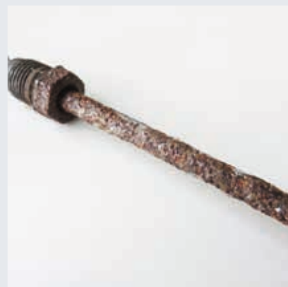
External damage, rust
