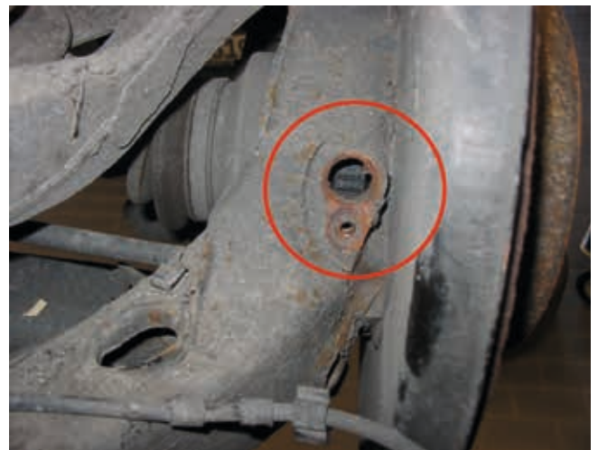
Check sensor installation point and impulse ring
